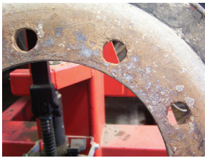
Debris trapped between wheels
